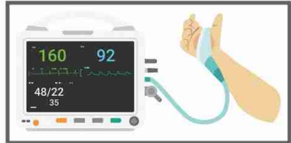
Figure 3.13. Pulse oximeter with sensor attached to a newborn infant's right hand on the hypothenar eminence.
