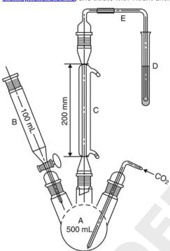
Figure 1. Apparatus for determination of sulfur dioxide.
